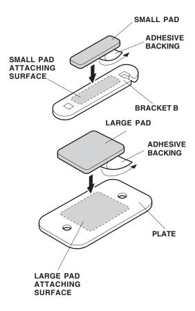
Using isopropyl alcohol on a shop towel, clean four plates where the large pads will attach.
